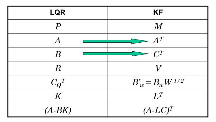
$LQR \qquad \qquad KF$   $[A, B] \text{ controllable} \xrightarrow{duality} [A^T, C^T] \text{ controllable}$   $KF \qquad [C, A] \text{ observable}$
