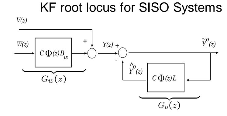
$$[1+G_o(z)] = [1+C\Phi(z)L] = \frac{\widehat{C}(z)}{\widehat{A}(z)} \quad \longleftarrow \quad \text{o.l. poles}$$
